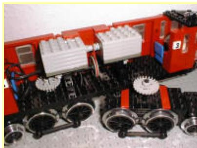
Mechanical power transmission of 4460. You can see two 9V motors driving a horizontal shaft by a rubber band. From here the speed is reduced once more to a third and with this speed the vertical shaft drives the wheel sets. The wheels are still using the original LGB metal shafts. The tooth gears are attached with help of some layers of tape to enlarge the diameter of the steel axle (see picture below). The electrical connection is shown more detailed in the next picture also.
